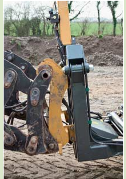
For front-mounting, the 1300 EH comes with an additional frame to sit between the handler carriage and the wrapper headstock. Control valve block (top) regulator wheels allow for fine-tuning of arm speed and roller speed.
