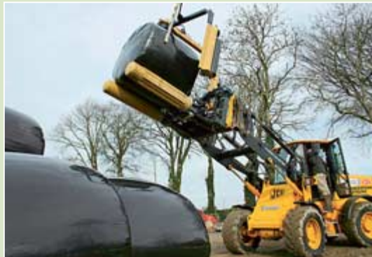
Wrapping can be commenced as soon as the bale is picked up and, in an ideal yard system, will be complete by the time the handler reaches the stack.
