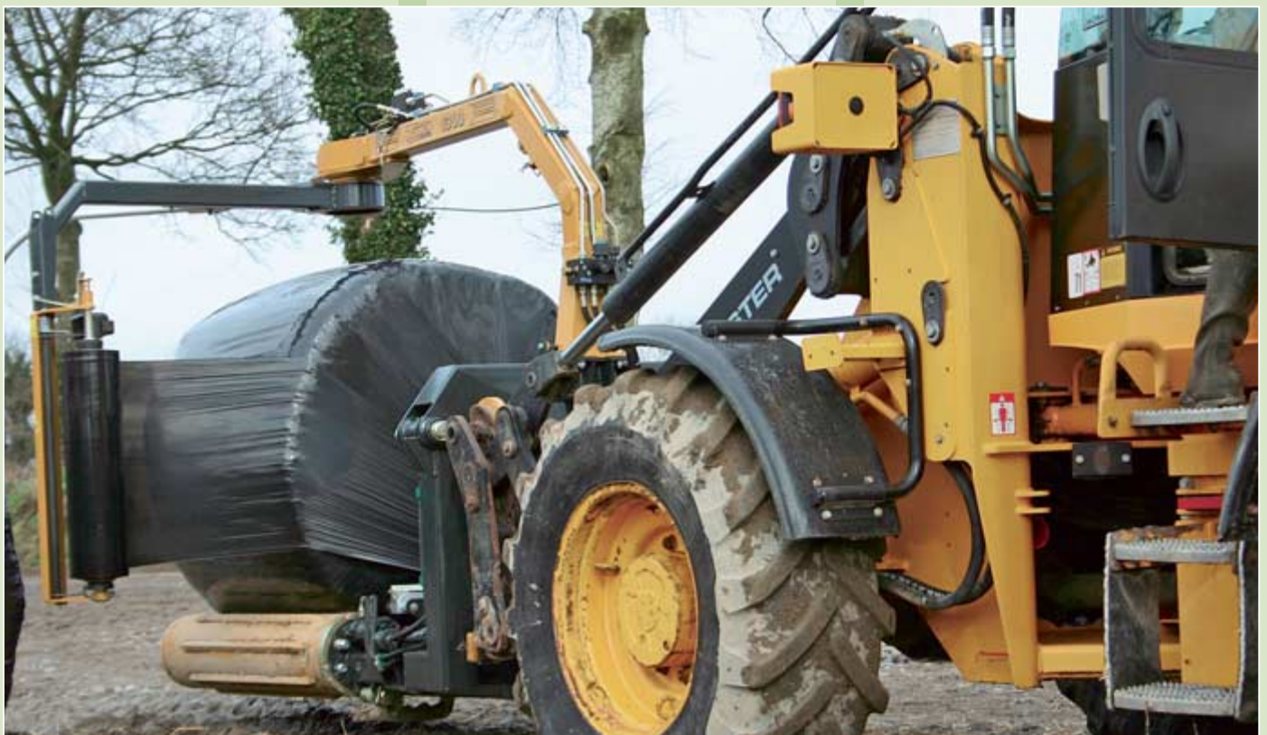
For front-mounting, the 1300 EH comes with an additional frame to sit between the handler carriage and the wrapper headstock. Control valve block (top) regulator wheels allow for fine-tuning of arm speed and roller speed.
