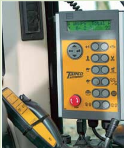
Remote control for roller operation can be 'married' to the handler joystick for one-handed control. The load/wrap/unload-at-the-stack technique is easy to master, a little nudging required to slot the bale into place.
