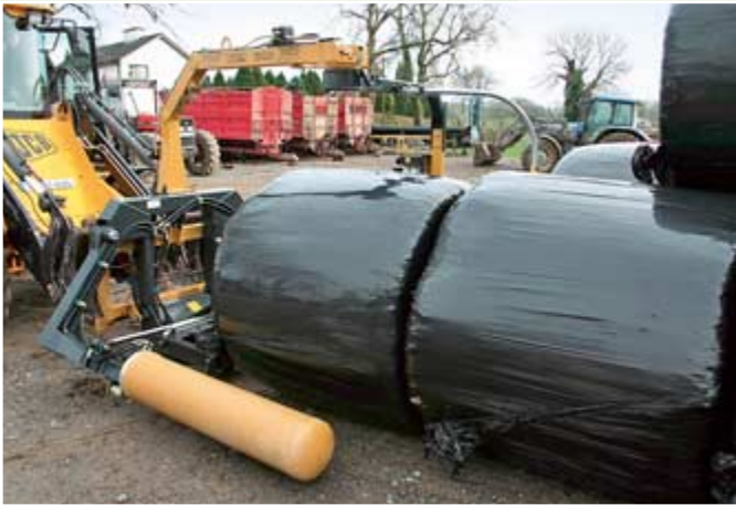
With the single satellite arm sited to the left of the wrapper when out of work, it's necessary to begin each bale row from right to left.
